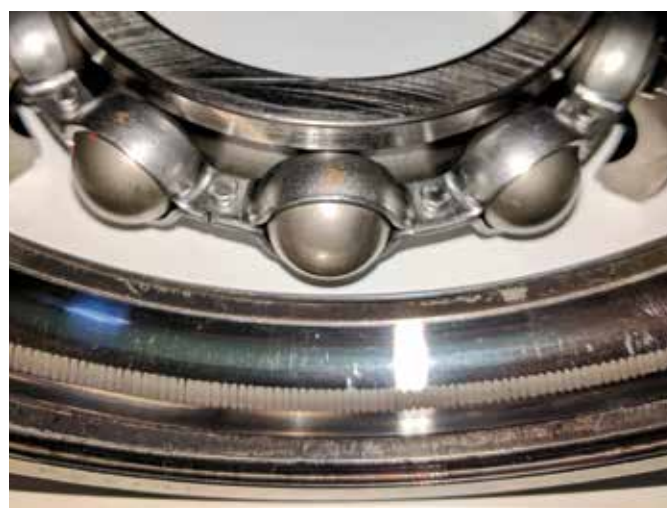
Photo: Striage dû aux courants de palier (Source: Dr. Hanna Putzi-Plesko, ZHAW School of Engineering)
