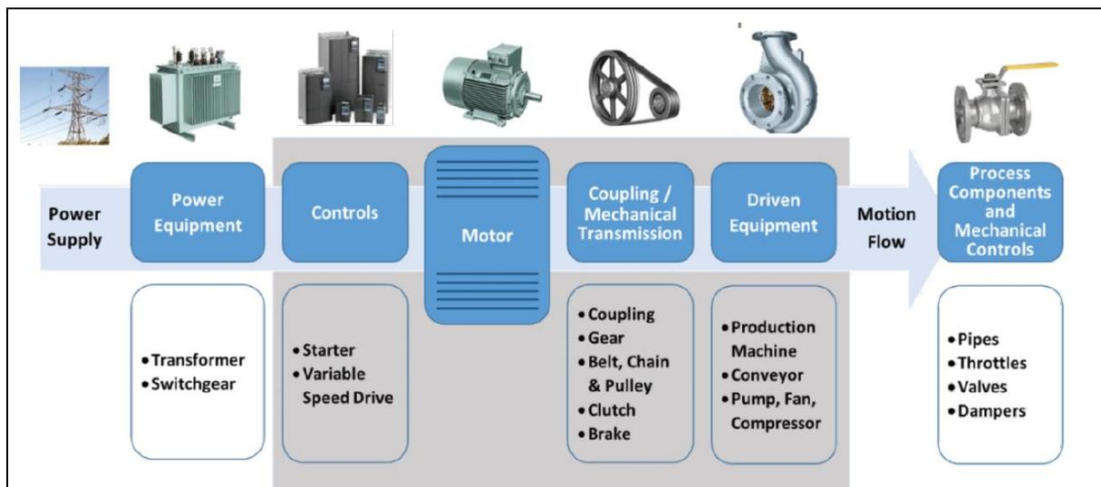
**Figure 1 The complete Electric Motor Driven System**
