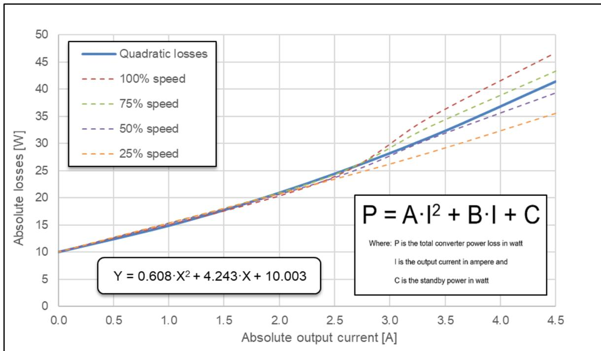
**Figure 4** Quadratic equation for curve fit of the relation between output current and losses
