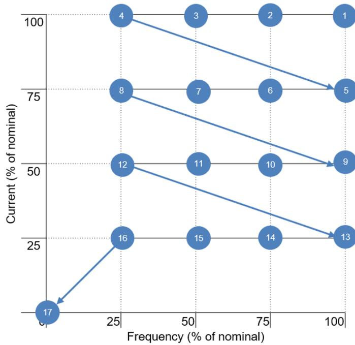
**Figure 3** 17 operating points of the converter tests according to the UTP in phase 1
