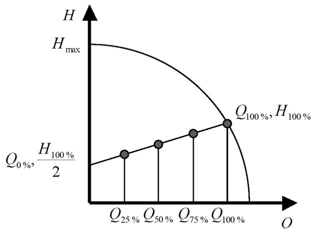
6. Select a setting of the circulator ensuring that the circulator on the selected curve reaches  $Q \cdot H = \max$  point.
